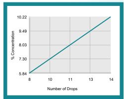
% Concentration = No. of Drops x Titration Factor Titration Factor = 0.73
