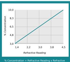
Concentration = Refractive Reading x Refractive Factor Coolant Refractometer Factor % Brix = 2,2
