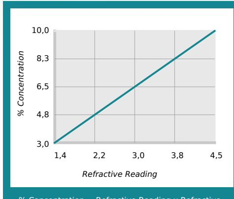
% Concentration = Refractive Reading x Refractive Factor
