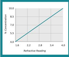
% Concentration = Refractive Reading x Refractive Factor Coolant Refractometer Factor % Brix = 2,5
