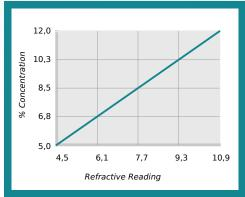
% Concentration = Refractive Reading x Refractive Factor Coolant Refractometer Factor % Brix = 1,1
