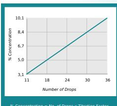
% Concentration = No. of Drops x Titration Factor Titration Factor = 0.28
