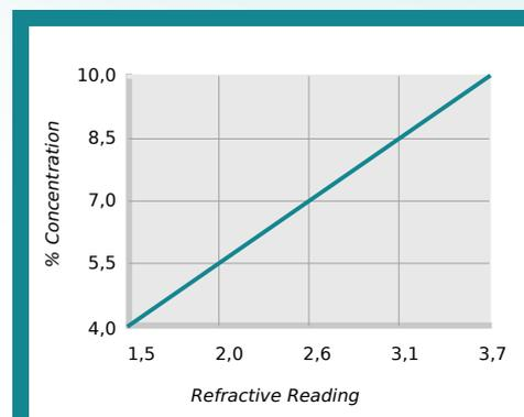
$\% \text{ Concentration} = \text{Refractive Reading} \times \text{Refractive Factor}$
