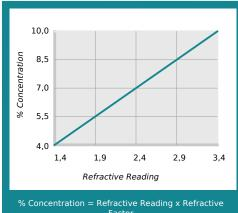
Coolant Refractometer Factor % Brix = 2.9
