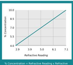
6 Concentration = Refractive Reading x Refractive Factor Coolant Refractometer Factor % Brix = 1.4
