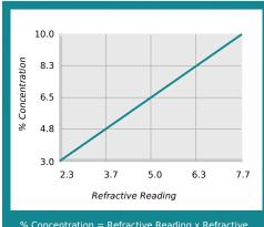
% Concentration = Refractive Reading x Refractive Coolant Refractometer Factor % Brix = 1.3
