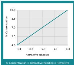
% Concentration = Refractive Reading x Refractive Factor Coolant Refractometer Factor % Brix = 1.2
