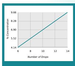
% Concentration = No. of Drops x Titration Factor Titration Factor = 0.69
