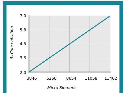
$$\% \text{ Concentration} = \text{Conductivity in Micro Siemens} \times \text{Factor}$$
