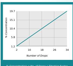
% Concentration = No. of Drops x Titration Factor Titration Factor = 0.58
