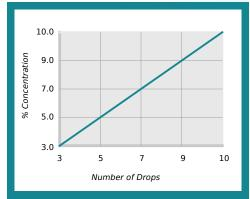
% Concentration = No. of Drops x Titration Factor Titration Factor = 1.00
