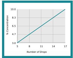
% Concentration = No. of Drops x Titration Factor Titration Factor = 0.59
