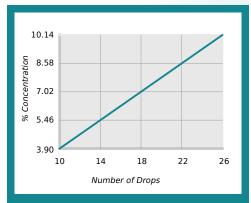
% Concentration = No. of Drops x Titration Factor Titration Factor = 0.39
