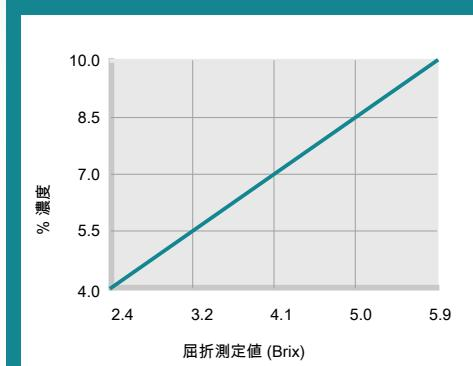
$$\text{% 濃度} = \text{屈折率測定値} \times \text{屈折係数}$$
