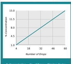
% Concentration = No. of Drops x Titration Factor Titration Factor = 0.25
