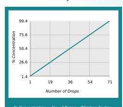
% Concentration = No. of Drops x Titration Factor Titration Factor = 1.40
