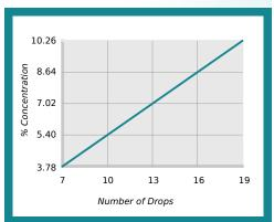
% Concentration = No. of Drops x Titration Factor Titration Factor = 0.54
