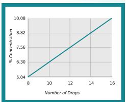
% Concentration = No. of Drops x Titration Factor Titration Factor = 0.63
