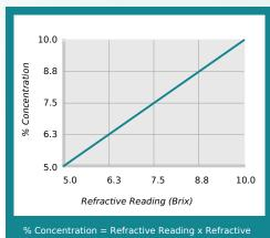
Coolant Refractometer Factor % Brix = 1.0
