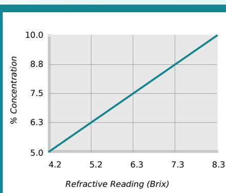
$\% \text{ Concentration} = \text{Refractive Reading} \times \text{Refractive Factor}$
