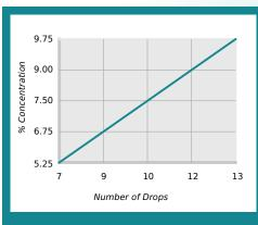
% Concentration = No. of Drops x Titration Factor Titration Factor = 0.75
