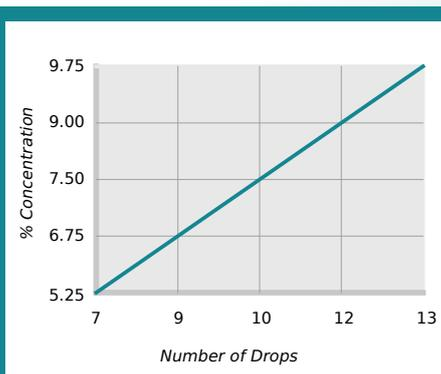
$\% \text{ Concentration} = \text{No. of Drops} \times \text{Titration Factor}$
