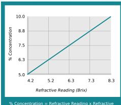
% Concentration = Refractive Reading x Refractive Factor Coolant Refractometer Factor % Brix = 1.2
