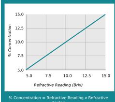
Factor Coolant Refractometer Factor % Brix = 1.0
