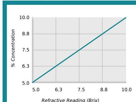
% Concentration = Refractive Reading x Refractive Factor
