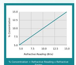
Coolant Refractometer Factor % Brix = 1.0
