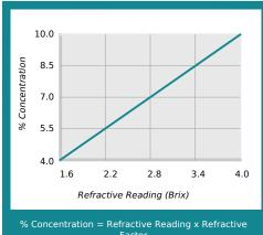
Concentration = Refractive Reading x Refractive Factor Coolant Refractometer Factor % Brix = 2.5
