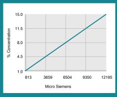
% Concentration = Conductivity in Micro Siemens x Factor Conductivity Factor = 0.00123
