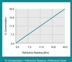
Concentration = Refractive Reading x Refractive Facto Coolant Refractometer Factor % Brix = 1.0
