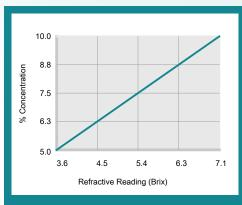
% Concentration = Refractive Reading x Refractive Factor Coolant Refractometer Factor % Brix = 1.4
