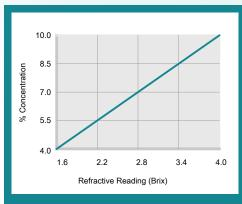
% Concentration = Refractive Reading x Refractive Factor Coolant Refractometer Factor % Brix = 2.5
