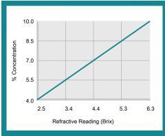
% Concentration = Refractive Reading x Refractive Factor Coolant Refractometer Factor % Brix = 1.6
