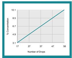
% Concentration = No. of Drops x Titration Factor Titration Factor = 0.18
