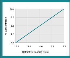
% Concentration = Refractive Reading x Refractive Factor Coolant Refractometer Factor % Brix = 1.4
