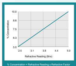
Coolant Refractometer Factor % Brix = 2.0
