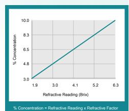
Coolant Refractometer Factor % Brix = 1.6
