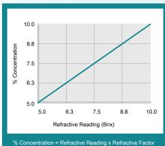
Coolant Refractometer Factor % Brix = 1.0
