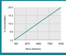
% Concentration = Conductivity in Micro Siemens x Factor Conductivity Factor = 0.00215
