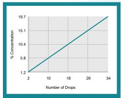
% Concentration = No. of Drops x Titration Factor Titration Factor = 0.58
