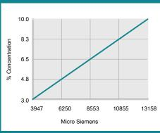
% Concentration = Conductivity in Micro Siemens x Factor Conductivity Factor = 0.00076
