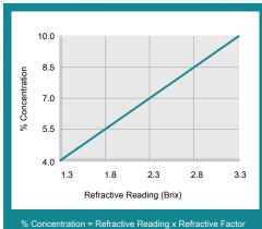
Concentration = Refractive Reading x Refractive Facto Coolant Refractometer Factor % Brix = 3.0
