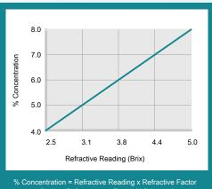
Coolant Refractometer Factor % Brix = 1.6
