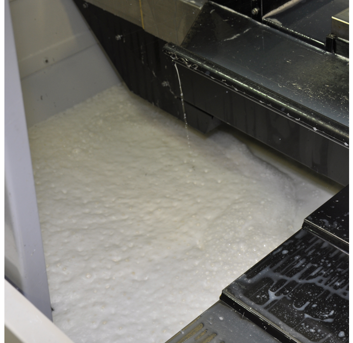
Foam in metalworking fluids can be a necessity or a major headache, with major headache winning out most of the time. Foam doesn't lubricate well, it cools poorly, it increases fluid volume, it adds to odor problems, and most importantly, it can damage machine plumbing.
