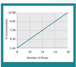
% Concentration = No. of Drops x Titration Factor Titration Factor = 0.63
