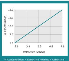
Concentration = Refractive Reading x Refractive Factor Coolant Refractometer Factor % Brix = 1.9
