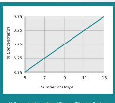
% Concentration = No. of Drops x Titration Factor Titration Factor = 0.75
