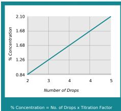
% Concentration = No. of Drops x Titration Factor Titration Factor = 0.42
