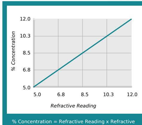
% Concentration = Refractive Reading x Refractive Factor
