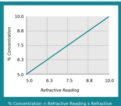
Concentration = Refractive Reading x Refractive Factor Coolant Refractometer Factor % Brix = 1.0
