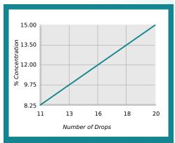
% Concentration = No. of Drops x Titration Factor Titration Factor = 0.75
