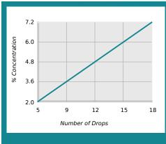
% Concentration = No. of Drops x Titration Factor Titration Factor = 0.40
