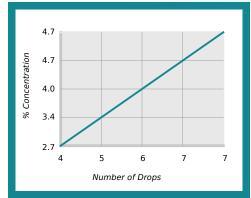
% Concentration = No. of Drops x Titration Factor Titration Factor = 0.67
