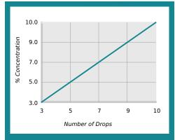
% Concentration = No. of Drops x Titration Factor Titration Factor = 1.00
