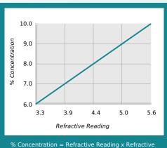
Concentration = Refractive Reading x Refractive Factor Coolant Refractometer Factor % Brix = 1.8
